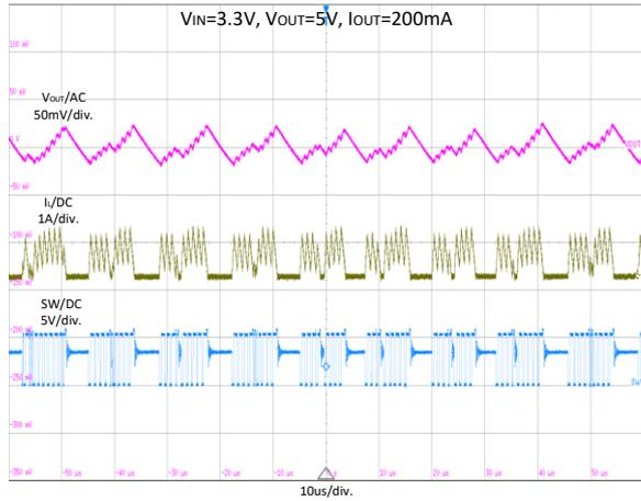
Figure 7. Output Voltage Ripple at Light Load
