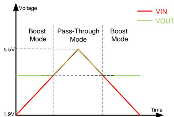
In the Boost mode ( $V_{IN} < V_{OUT\_SET}$ ), and the boost converter switching, the ET8290B features reverse current blocking capability, which prevents voltages higher than  $V_{OUT\_SET}$  from leaking back to the VIN pin. However, in Pass-Through mode, VOUT does not have reverse current blocking functionality.
