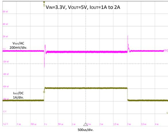
Figure 13. Load Transient
