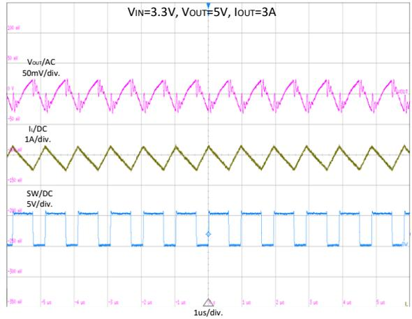
Figure 8. Output Voltage Ripple at Heavy Load
