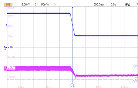
200us/div, V_{OUT}=5.0V I_{OUT} = 1A V_{IN}=17V to 6.5V Figure40. ET8123 Line Transient
